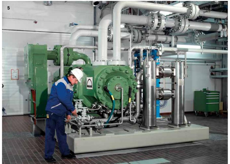
**5** The tandem HOFIM™, offers the added capability of operating the two casings either in the series or in the parallel modes. This allows the operator to cover the widest possible duty range at high efficiencies. Switching from one mode to the other can be effected during operation without shutdown.
