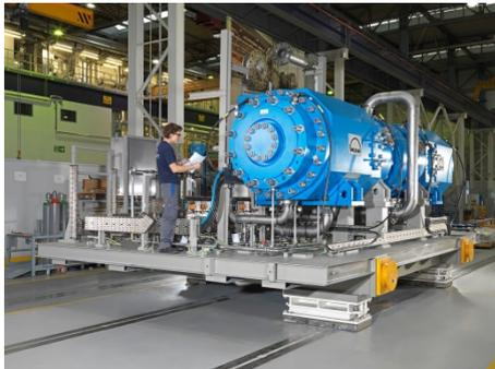
The hermetically-sealed HOFIM™ motor-compressor system for Ivar Aasen
