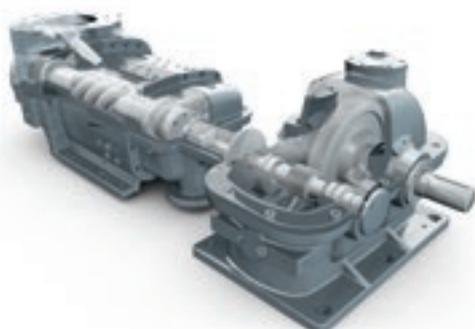
The SKUEL series is available with five different rotor diameters, each with two different length-to-diameter ratios. Suction flow rates are available between 4,000 m³/h and 100,000 m³/h with discharge pressures up to 16 bar. A horizontally split casing design allows ease of maintenance.
