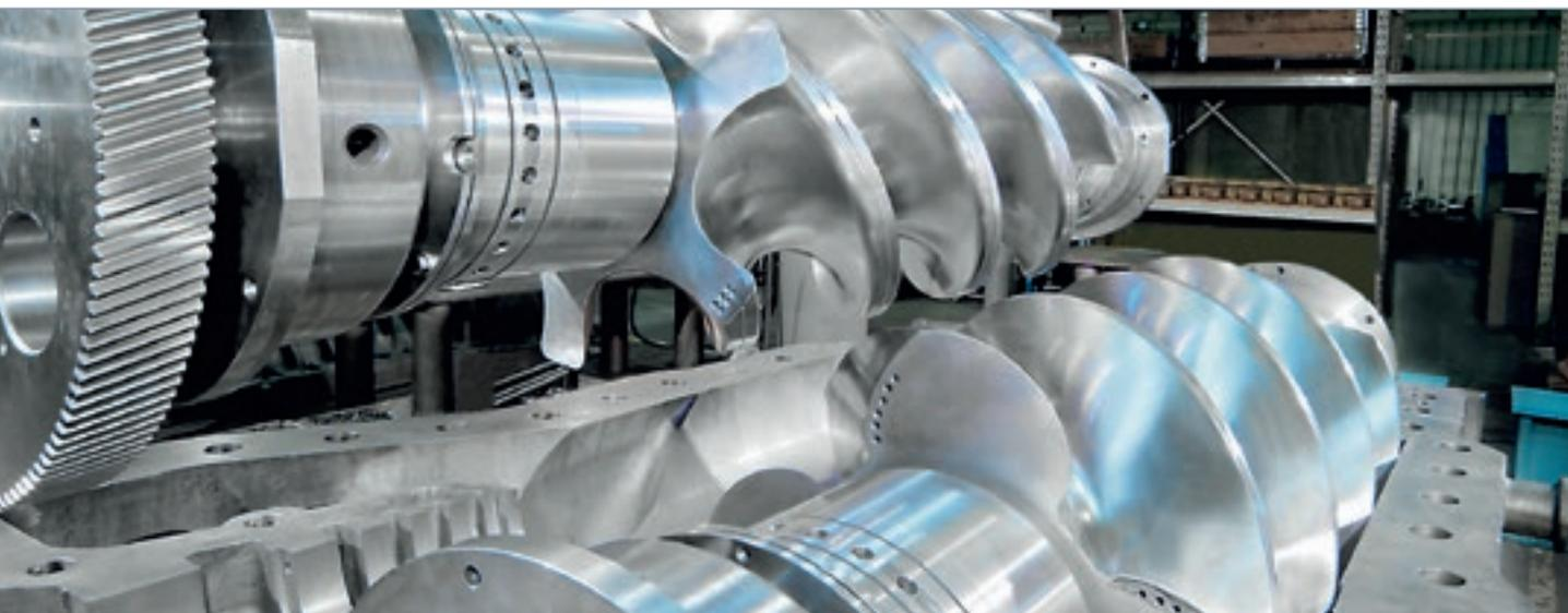
1 Large-scale rotors of SKUEL type screw compressor
